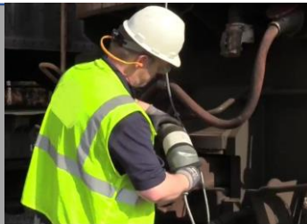
MU-Kit cable connects from the MU receptacle to the test console
