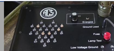
... and verifies the lights that correspond to the appropriate pins are illuminated on the test console
