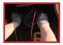
With ACS-RS MU Test Kit, a single electrician plugs the cable into the receptacle and uses console to complete the test in the cab
