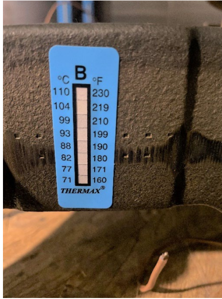
Figure 6. Bearing adapter after 60 temperature cycles
