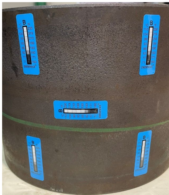
Figure 10. Bearing cup after reaching 180°F (View 1)
