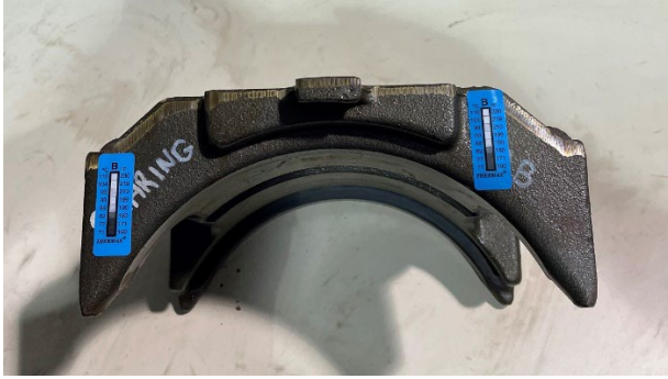
Figure 8. Readability of bearing adapter after reaching 180°F (View 1)
