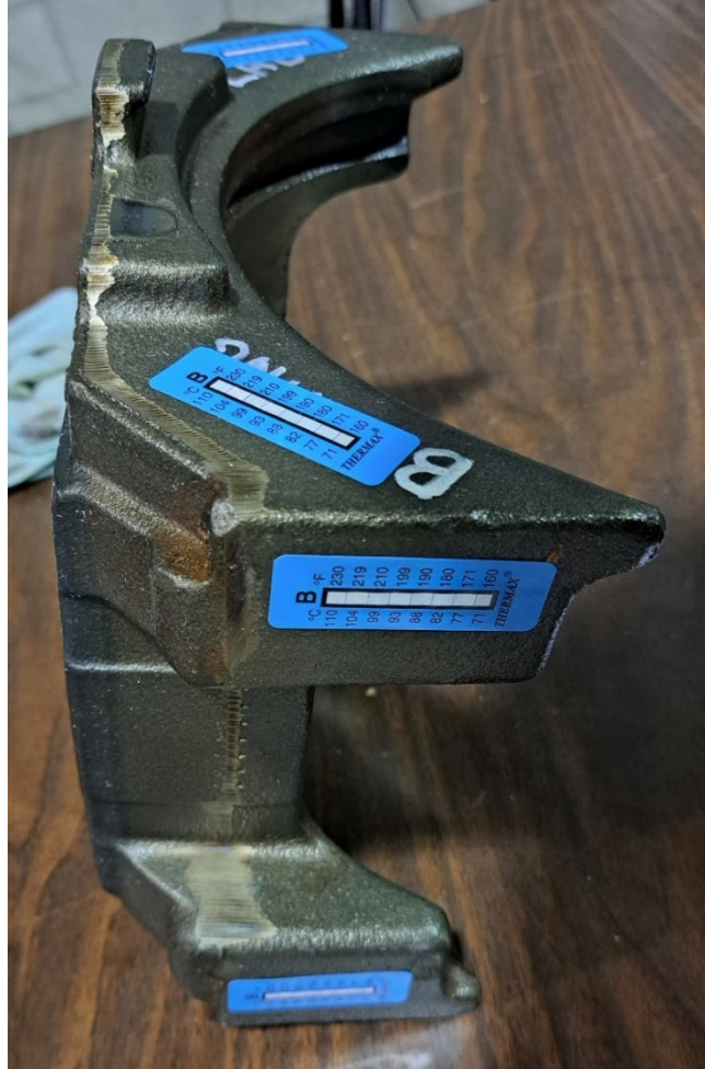
Figure 4. Bearing adapter with indicator strips
