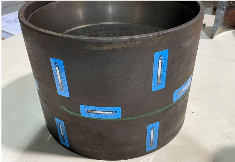
Figure 11. Bearing cup after reaching 180°F (View 2)
