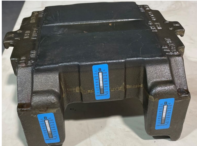
Figure 9. Readability of bearing adapter after reaching 180°F (View 2)
