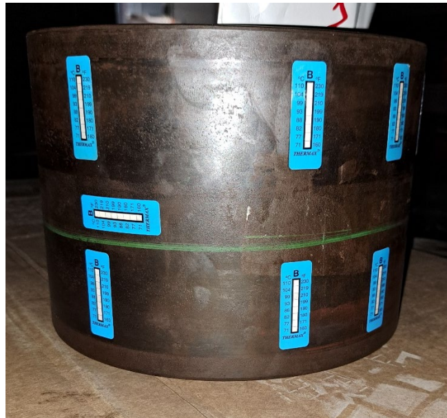
Figure 3. Bearing cup with indicator strips
